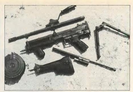
Ultimax 100 SAW - disassembled.
